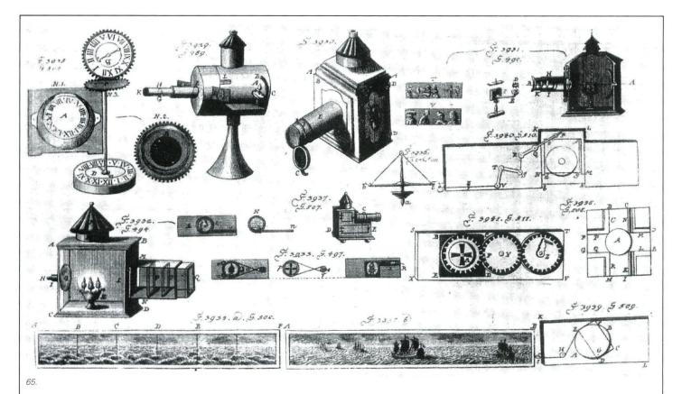
**No. 3930** shows another magic lantern from Denecke in 1757, as No. 3922 above. This lantern already has a lens cover, and Denecke reported that 'The picture which this lantern gives, in its ordinary distance from the wall, is about as big as a middle-sized wagon wheel.'
