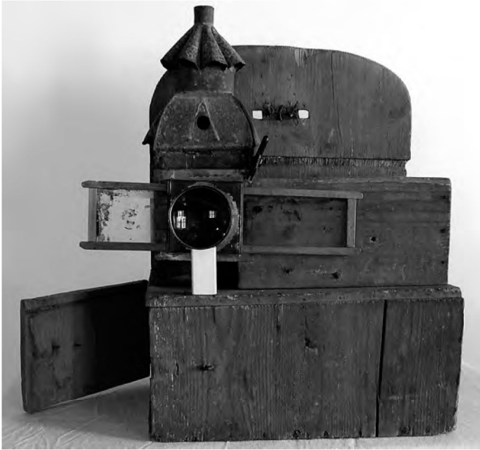
4. The lantern set up as though for projection, with the lens and slide carrier from another lantern temporarily held in place by a clamp
