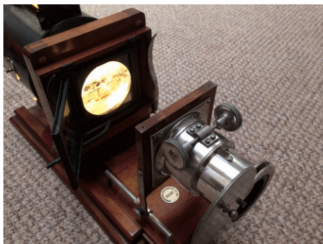
7. The 'double-action flap changing device' in action. (a) stage 1 (b) stage 2: mid change (c) stage 3: new slide appears with audible 'flack'
