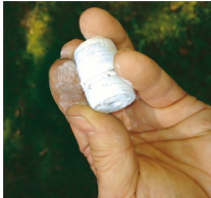
4. Homemade lime cylinder just cut from marble
