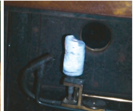
5. Eroded lime after use
