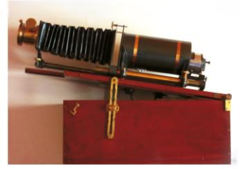
too much adjusting. The correct focusing could be done by moving the bellows on a tubular rod with a single screw to hold it in position, and adjusted to any angle to suit the screen. The whole lantern and base-board could be turned upside down and secured inside the case, with a handle for carrying.
