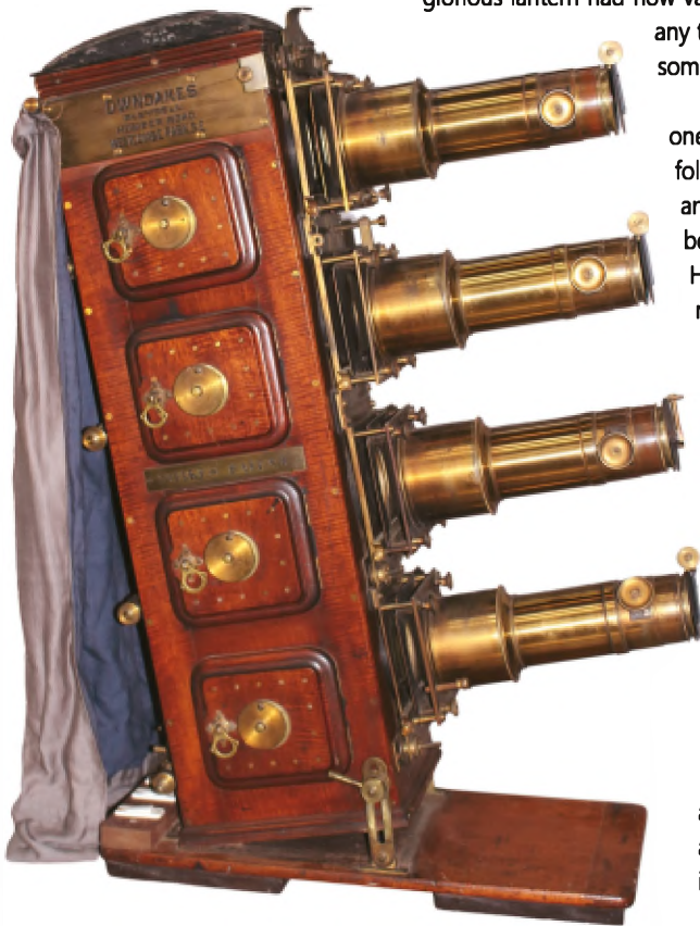
2. The Noakes Quad lantern, right profile, with the lens extension tubes in place and the body tilted back to the full extent
