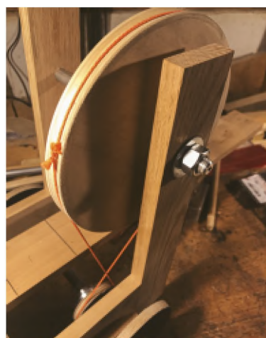
2. Work in progress – building up the gear for the rotating cam axle
