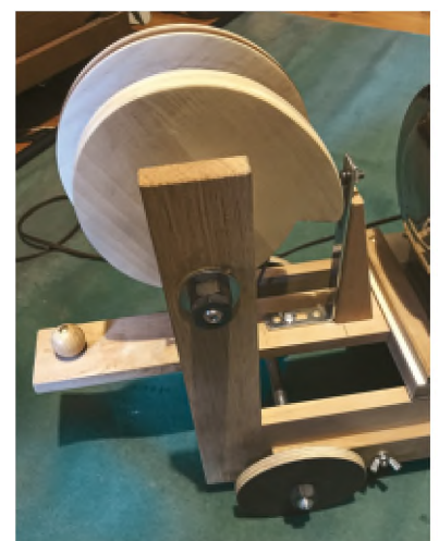
4. The cam in the position with maximum bellows extension
