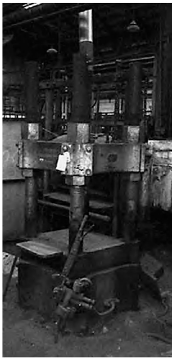
2. Surviving Woodburytype press found in the former Eveleigh Locomotive Works in Sydney (reproduced, with thanks, from the Woodburytype Resource Site, www.geocities.com/woodburytype )
