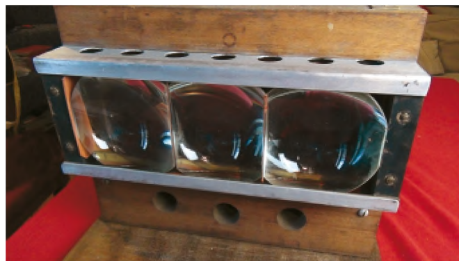
4. The three condensers, cut vertically to align with the photographs, light sources and lenses
