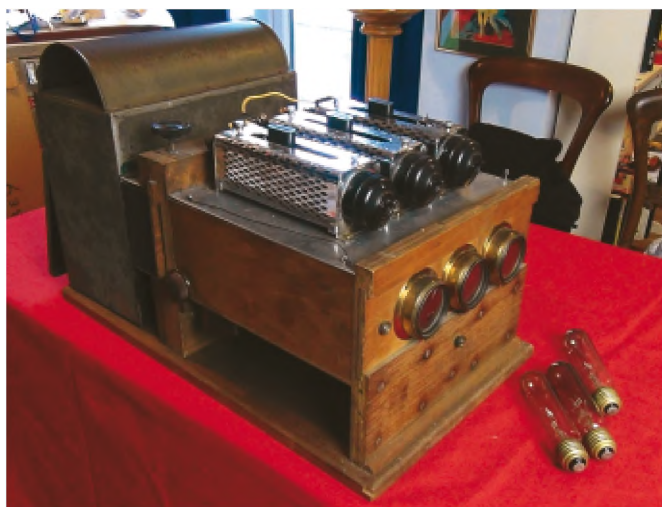
2. After cleaning up, with the original Edison lamps, marked 30V 250W
